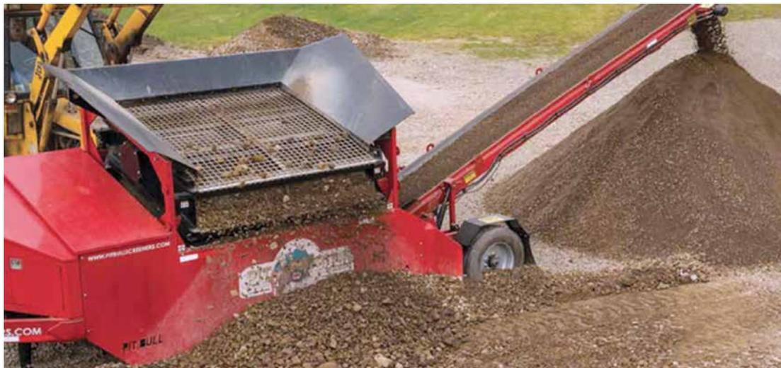
Simply loosen the four tension bolts on the loading side of each tier and the operator can switch out their screens in less than 30 minutes. Unlike any other screener on the market, the Pitbull 2300 Screener has the ability to reverse the screen direction to easily break up stubborn material.
