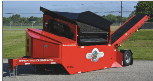
The Pitbull portable screening plant with conveyor can process 1 cu. yd. (.76 cu m) of material under good conditions every 23 seconds.
