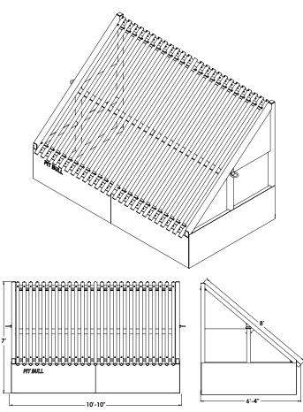
Our PB106 stands 7 feet at its highest point and can stand up to the toughest material, from coarse gravel to demolition debris.
